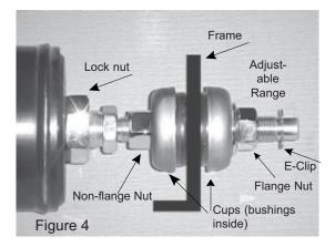
Mount the rear eyes of the shocks using and washers, and tighten all shock mounting hardware to the proper torque specifications (see shop manual for specs). Route the adjuster line in a seeping arc above the right shock and toward the rear (fig.5).
