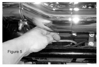
■ Route the line up and then to the left side of the bike. As you do so, make sure the line will not be pinched, kinked, or exposed to excessive heat and use the included zip-ties to secure it in place. Route the line out the left side in front of the fender and above the lower belt-guard (fig.6).
