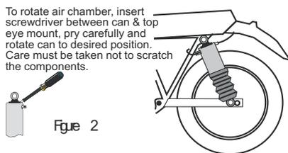
B. Progressive shock absorbers are mounted in the same location as the stock shocks.
