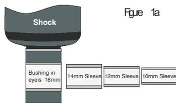
1. With the exception of the shock mounting sleeves (See figure 1a), it is mandatory that the shock absorbers not make contact with any part of the motorcycle. Damage can result if they are not mounted with adequate clearance (See Figure 1b).
