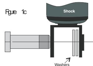
Eye To Clevis Mounts: On clevis mounted shocks, no clearance is necessary. If clearance exists, install washers (supplied) to remove clearance (See Figure 1c).
