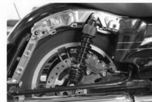
5. Set your ride sag. The proper spring pre-load setting will permit the rear suspension to sag, or compress, approximately 1/3rd of the total available wheel travel from full extension. To make this simple, fast and easy;
