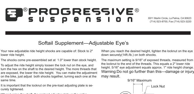
When turning the shaft, the preload adjuster plate or the entire spring housing may turn along with the shaft, this is ok, it is not changing your preload setting.
