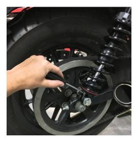
**Increase Rebound:** More rebound may be desired if the back of the bike feels like it is kicking up too much during braking or after a bump is hit. More rebound may also be desired if the bike feels like it is moving around excessively and not settling down after hitting a bump.
