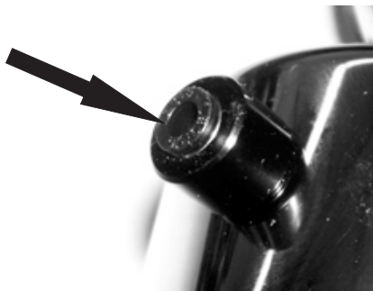
Photo 2 - Push in the collar to remove the plug or air lines.
