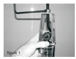
3. Crank the handle clockwise, which will start to pull the upper eye up and out of the spring (and cover if equipped).
