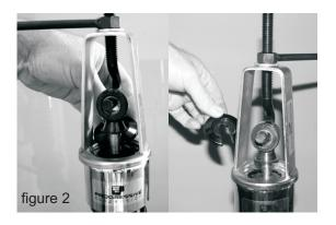
5. Once the spring retaining clip is removed, carefully crank the spring tool counter-clockwise to release the spring pressure. Keep cranking until all the spring pressure is gone and the tool is loose (see figure 3).
