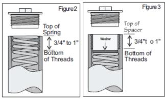
Also check the Notes in the enclosed Application Supplement, the stock spacer in some cases can be modified to fit. If making a spacer, we recommend PVC pipe that is the approximate diameter of the fork springs but will still fit inside the fork tubes. *Warning:*
