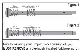
**MUST REMOVE** any previously installed fork lowering kit components, such as the 1 or 2 additional top out springs illustrated above. Additional top out springs are common in many such kits.
