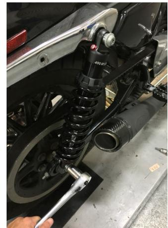
**4.** Reinstall any accessories removed in accord with their mounting instructions. Make sure accessories do not interfere with the shocks throughout their full travel. If any accessories bolt to the shock mounting points, a careful inspection must be made to insure that they do not bind the shocks in any way. Your shocks will come pre-installed with either bushings or bearings; refer to your hardware pack supplement during installation.
