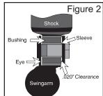
B. If excess bottoming occurs, adjust cam to a
